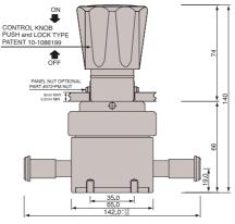
For 1/2" Model 2MS and 2FS 142mm For 1/2" Model 2ML and 2FL 180mm For 3/4" Model 3MS and 3FS 160mm For 3/4" Model 3ML and 3FL 000mm
