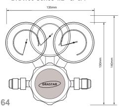
For 1/4" 4MS and 4FS Model 94mm For 1/4" 4ML and 4FL Model 000mm For 3/8" 8MS and 8FS Model 120mm For 3/8" 8ML and 8FL Model 000mm
