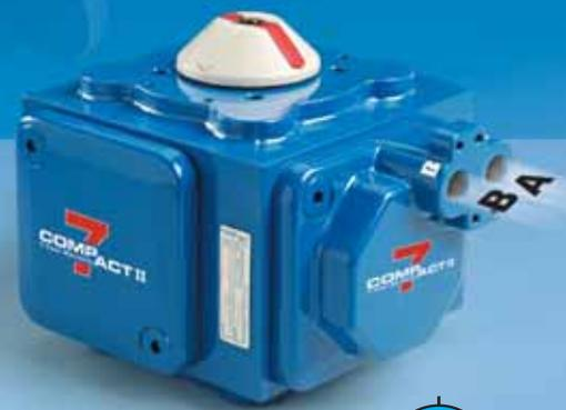
The **COMPACT II** actuator transforms the linear motion of its pneumatic pistons into rotary motion via 4 gear racks that drive the central pinion. Air Supply, to drive the pistons, flows into port **A** of the NAMUR cover: Port **A** is connected to the center chamber and port **B** is connected to the four outside chambers.
